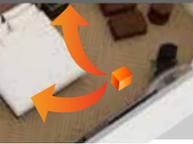
Place the heater and additional ventilators as shown in the diagram to ensure the right airflow. Adjust the position of the heater to maximize the airflow according to the configuration of the room.
